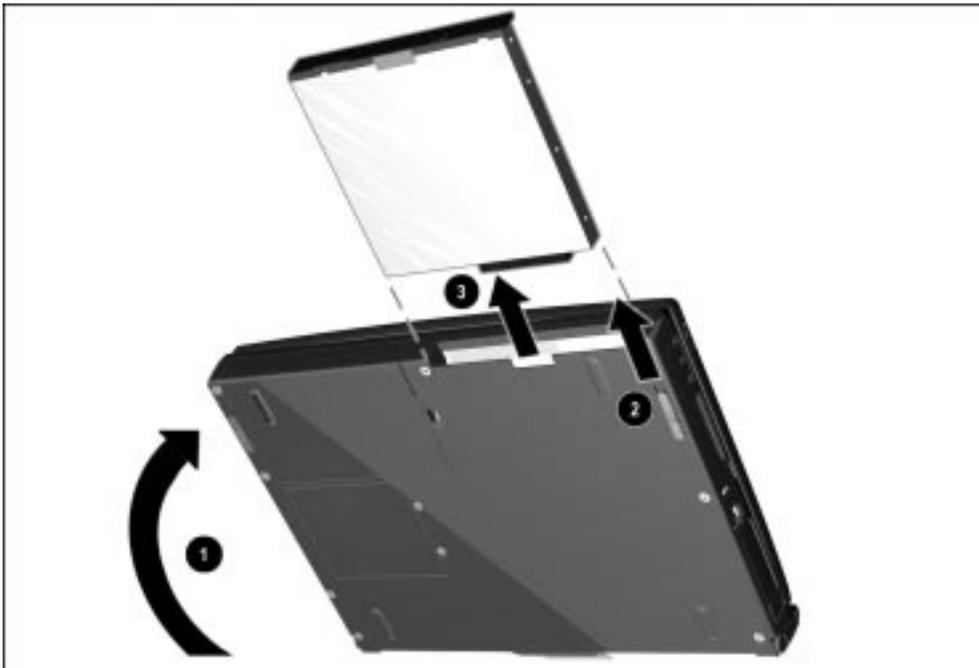
*Figure 5-12. Releasing a Device from the MultiBay*
