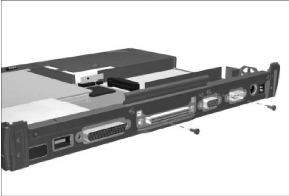
*Figure 5-42. Removing the U-channel Screws*
