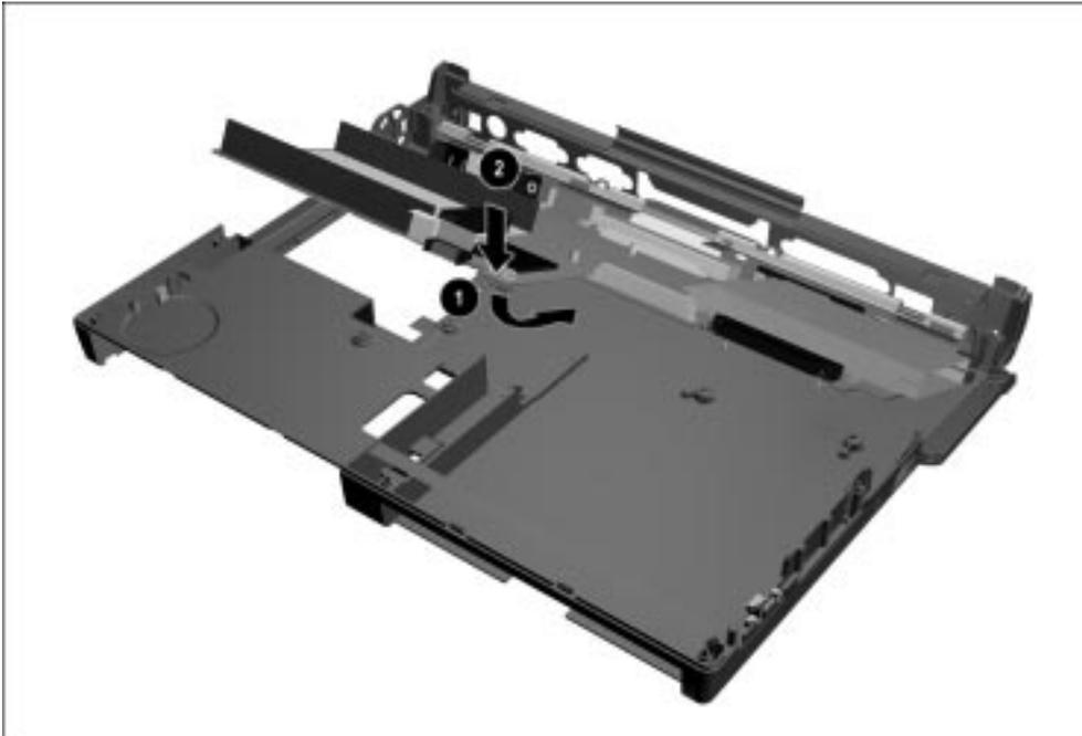
*Figure 5-45. Installing the System Board*
